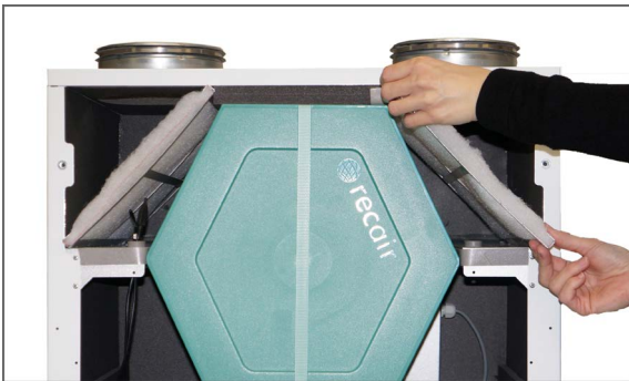
3. Remove the two filters from the unit.
